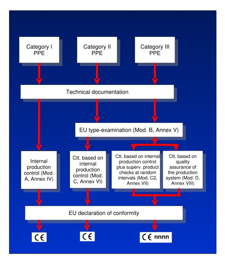
For Category II and III PPE, before serial production starts, the model (type) of the PPE has to be submitted for an EU type-examination. Exceptions are pre-prototypes and research prototypes.
